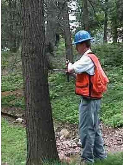
Fig. 10.8 The forester inserts the increment borer by turning the threaded tip into the tree.
